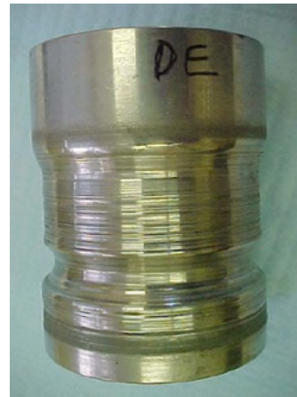
Hardened 420SS sleeve wear after 3 weeks
